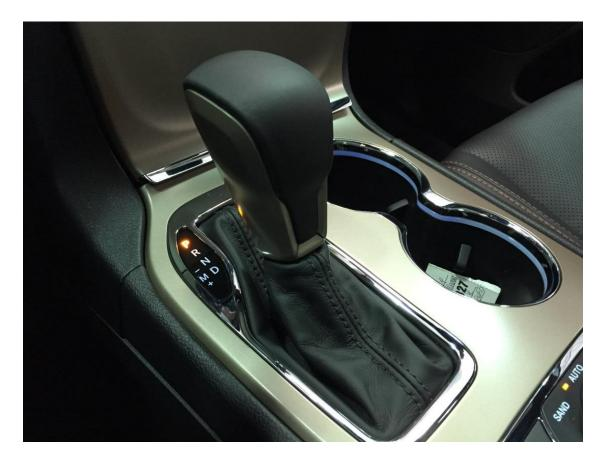
141. As the above image demonstrates, the Polystable Shifter slides back and forth and rests in predetermined physical slots for P, R, N or D.
